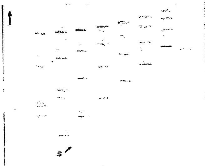
Fig. 5. One-dimensional separation of a mixture of 21 amino acids on a silica gel 60 F 254 HPTLC plate. Solvent, n -butanol–acetic acid–water (4:1:1); continuous development; running time, 70 min; flow-rate of solvent, 10 cm 3 /h; external pressure on membrane, 1.2 MPa; marker substances at layer's edges; s 0 (start distance) increases diagonally.
